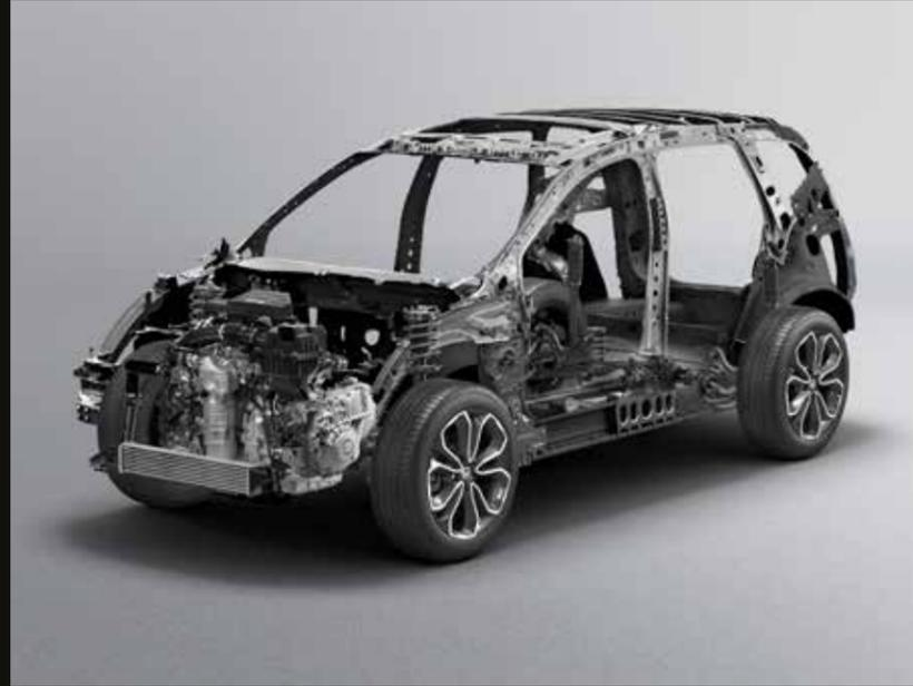
As an integral part of the CR-V structure, Honda's Advanced Compatibility Engineering™ (ACE™) body-structure enhances occupant protection and crash compatibility in frontal collisions by distributing crash energy more evenly throughout the front of the vehicle.
