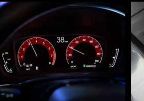
**Full-color LCD panel:** The All-New Civic features first all-digital LCD instrument display. Measuring 10.2 inches, the high-definition full-color LCD panel displays a variety of information, all customizable from the steering wheel.
