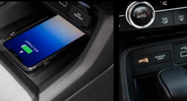
**Wireless Charging:** Phones supporting wireless charging can be easily charged, using the Wireless charging platform in the center console.
