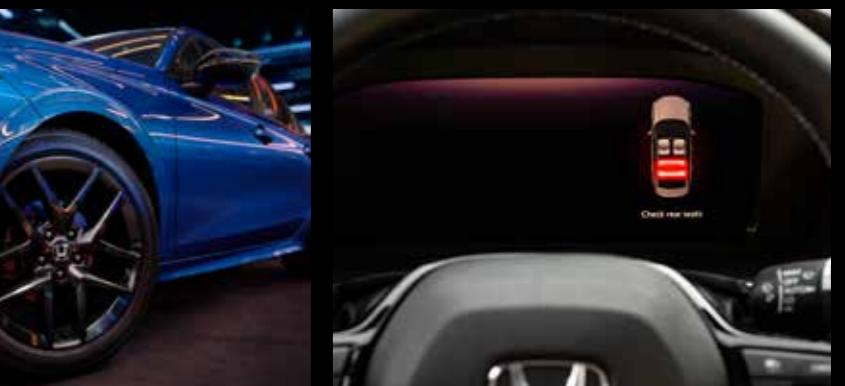
**Honda LaneWatch™:** Honda LaneWatch™ uses a camera installed below the right passenger-side mirror to relay an image of the area on the right side of the vehicle to the central display screen with the wide angle views.
