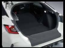
This reversible, foldable boot mat offers protection to your boot and to the complete loading floor when the rear seats are folded down.
