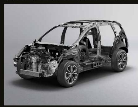
As an integral part of the CR-V structure, Honda's Advanced Compatibility Engineering™ (ACE™) body-structure enhances occupant protection and crash compatibility in frontal collisions by distributing crash energy more evenly throughout the front of the vehicle.
