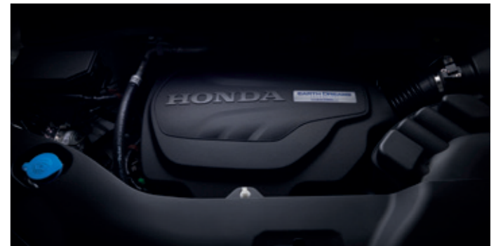
3.5-liter direct injected i-VTEC® 24-valve SOHC V6 engine
