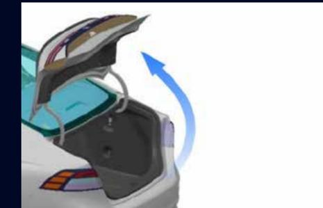
Lid raises automatically when the trunk is opened for easier access when loading or unloading cargo.
