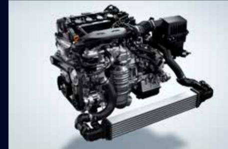
The 1.5 liter VTEC Turbo produces 194 hp and 260 Nm of torque from 1,700 rpm for instant response.
