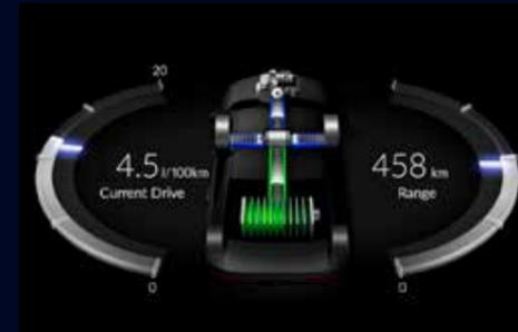
Engine drive sends power directly to the wheels to maintain continuous higher speeds, for example on highways, while charging the battery at the same time.
