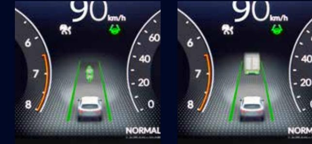
The TFT meter can show vehicles detected whilst in ACC mode, with real-time data.
