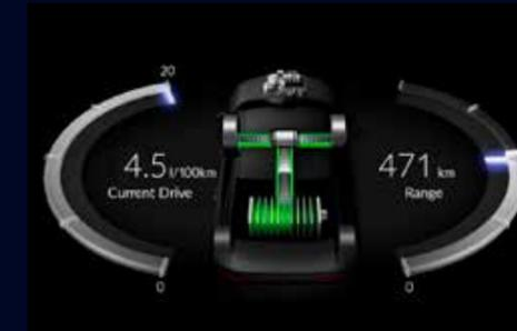
With regenerative braking, energy discharged when you apply the brakes is returned via the charge motor to top-up the high voltage battery.
