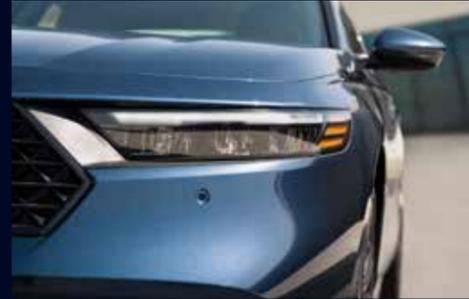
The Accord's simple, uncluttered appearance has been achieved by integrating many of its external features. The front radar sensor is contained in the Honda badge and wedge-shaped headlights are integrated with into the grille with precision form and unity with the bumper. The new dual low-beam design with darkened housing gives the headlights a dramatic look, day or night.
