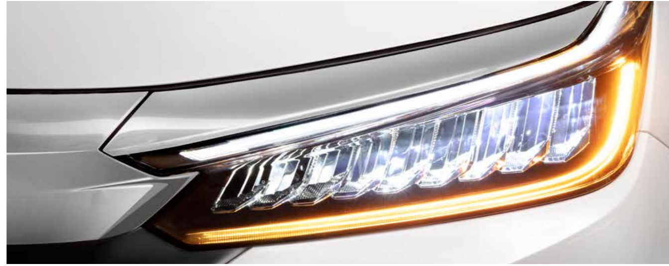
Full LED headlights with 9 LED array Inline shell, integrated LED DRLs and L-shaped LED turn signals.
