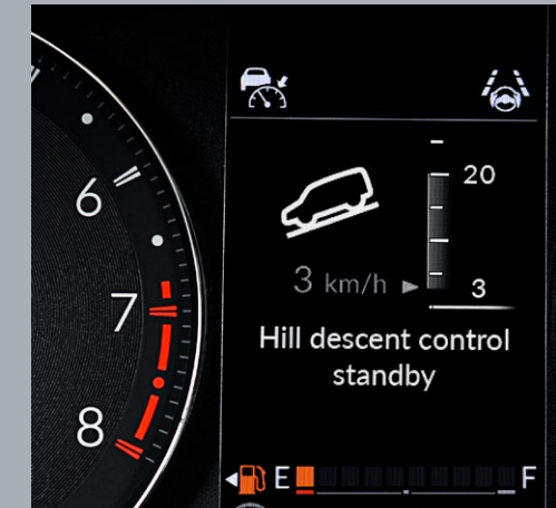
Hill Descent Control (HDC), automatically controls the speed between 0-20 kmph when descending hills
