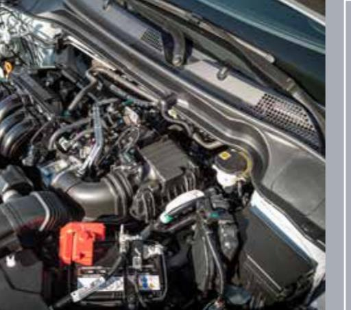
1.5L DOHC i-VTEC Engine with Continuously Variable Transmission (CVT)
