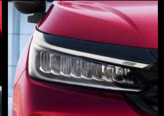
Integrated LED Daytime Running Lights (DRLs)
