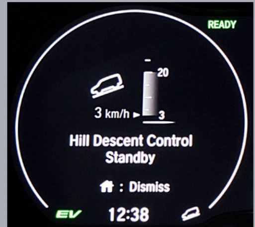
Hill Descent Control (HDC), automatically controls the speed between 0-20 kph when descending hills
