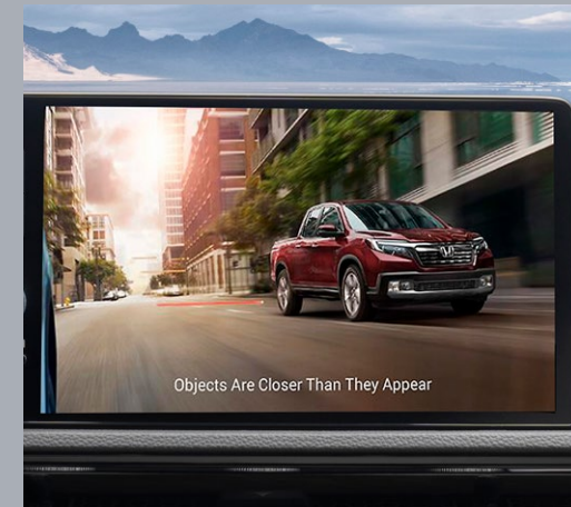
LaneWatch™ gives the driver a clear image on the audio screen, of any vehicles in the blind spot
