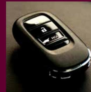
Press the tailgate button on the key fob to open the tailgate.
