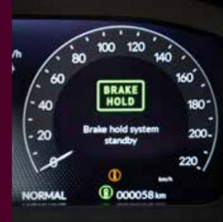
**Electronic Parking Brake with Brake Hold**
